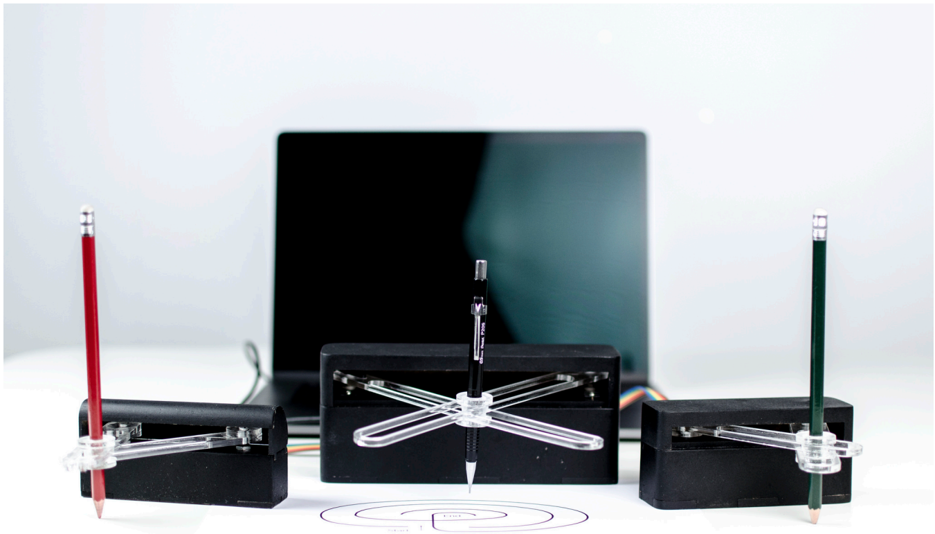
Figure 4, The drawing machine. The drawing hub is in the centre, flanked by two drawing nodes.
