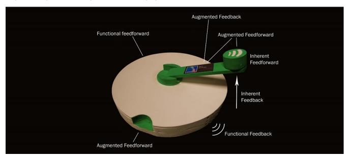
Above is an overview of feedback and feedforward in SPOT. SPOT looks like a record player and has very obvious speaker holes conveying it is a music player. The lever nearly screams to be lifted, and reveals the other functions SPOT offers when it is brought to an "on" state.
